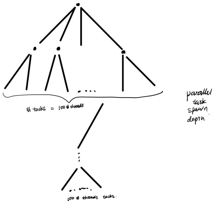
With one level of task spawn, in the most extreme case, only one out of the many tasks is non-trivial. This task may be given to a thread and the other threads are simply waiting for it to perform sequential algorithm. We can reasonably expect the speedup from this scenario to be abysmal. Note, this imbalanced subtree property of IDA is eventually limiting to the overall speedup. (We will discuss in further details in the Results and Analysis sections).
