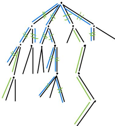
For example, in the above graph, iteration  $i$  may be traversing the tree over blue edges with no solutions found. Then, iteration  $i + 1$  may traverse with blue plus green edges.
