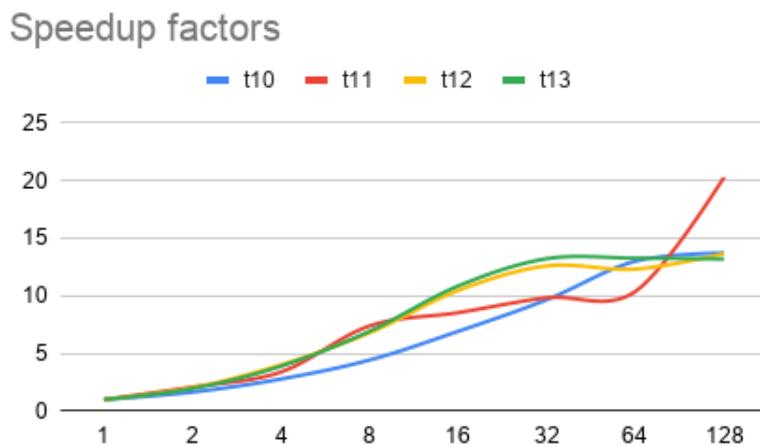
Note that it may appear that scaling has slowed down, but notice for t11, the scaling at num\_threads = 128 is great. This measurement is persistent, and we provide a detailed explanation below in the analysis portion, as for why the scaling factor is not always linear, or may even appear to be inconsistent (i.e. in the t11 case) or superlinear.
