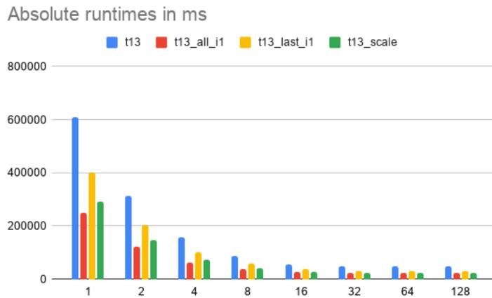
We can observe that, as expected, the absolute time in terms of execution is the lowest for `t13_all_i1`, next lowest for `t13_scale`. Next that `t13_scale` is still much faster than `t13_last_i1`, since the solution step from  $S_1$  is much higher up in the search tree.
